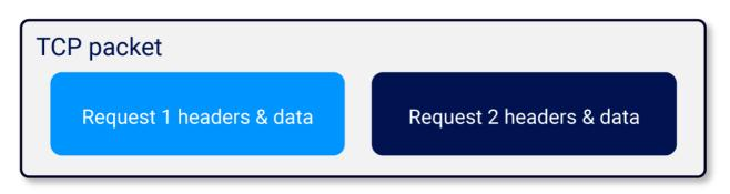
This is a novel possibility with HTTP/2 because it allows HTTP requests to be sent over a single connection concurrently, whereas in HTTP/1.1 they have to be sequential.
