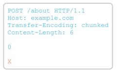
Thanks to the terminating '0' chunk the front-end will only forward the blue text, and the back-end will time out waiting for the X to arrive.
